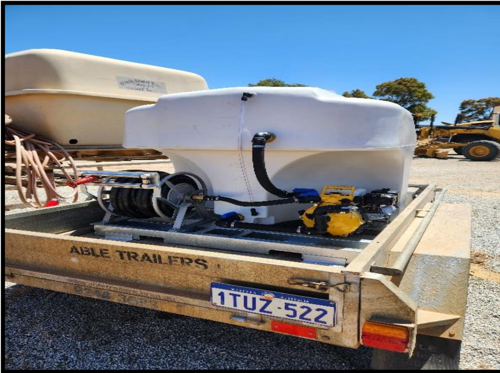
The new skid mounted fire tank set up on the trailer.
